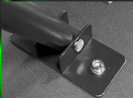
Step 4: Secure the support pole bracket to the lamp body.
